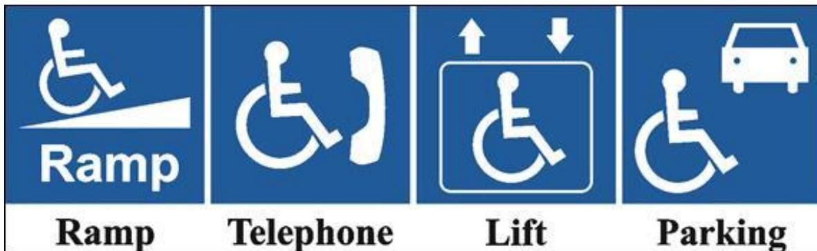
Figure 6-29: Signage for Accessible Facilities
